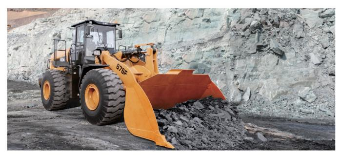
The 676F is highly versatile and suitable for a wide range of applications, including the loading of aggregates and bulk materials, coal, various types of rock, ores, and more. Aligned with SEM's commitment to high reliability, the 676F incorporates upgraded drive and hydraulic designs, ensuring superior reliability, efficiency, straightforward operations, and swift hydraulic motions.
