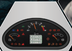
FAULT CODE IN CLUSTER
